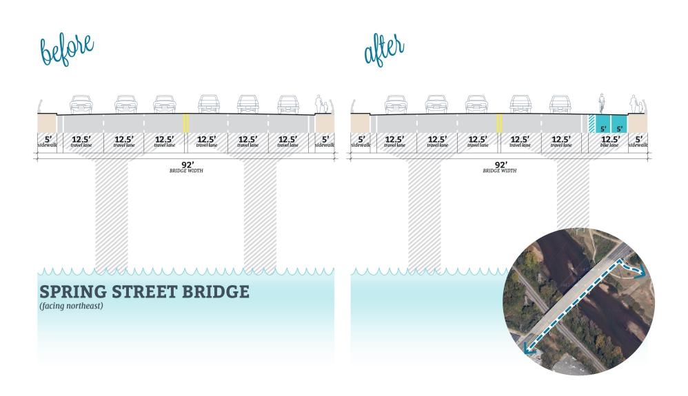
Spring Street Bridge Option 1; remove one lane of traffic and provide a buffered bikeway on the East side of the bridge.
