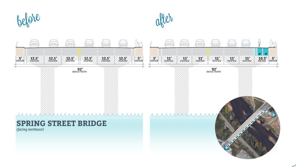
Spring Street Bridge Option 2; keep the same number of lanes but narrow them to 11' and provide a buffered bikeway on the East side of the bridge.
